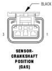
Figure 26 - Crankshaft Position Sensor Connector Pinout
