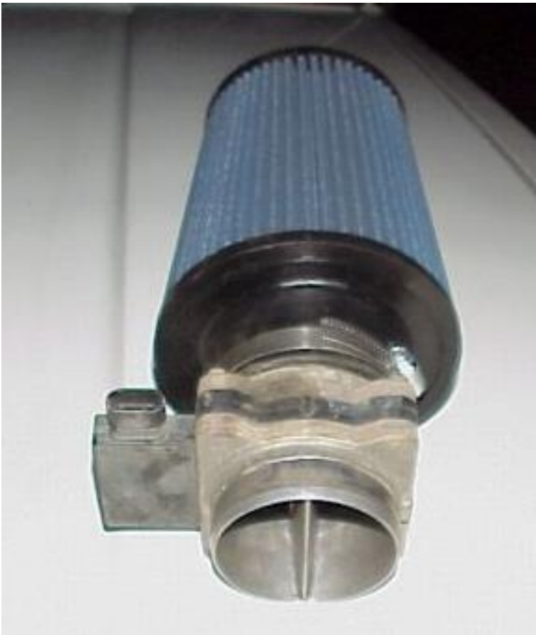
Figure 5 - MAF sensor with air filter fitted.
