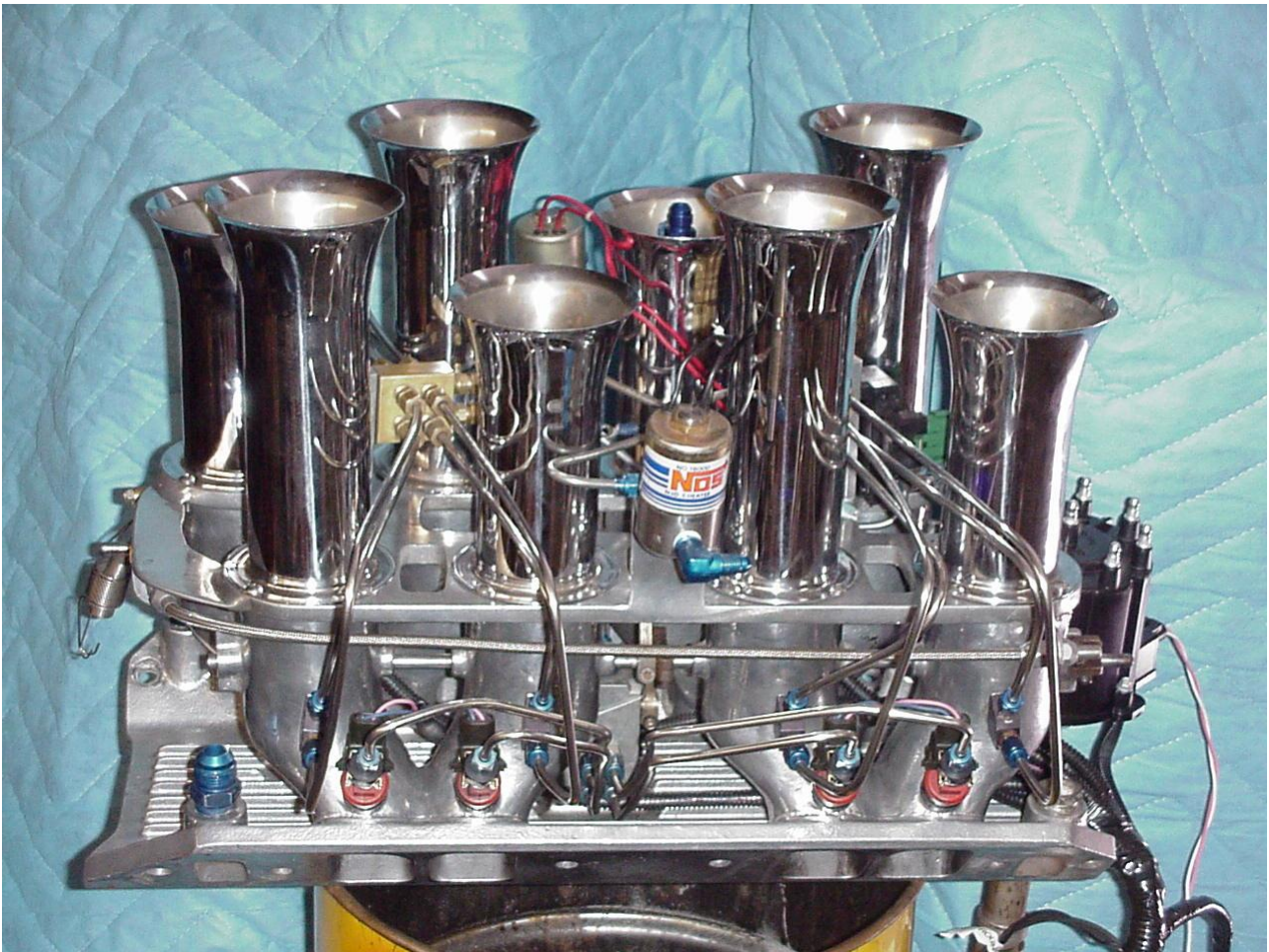
Figure 5 - Big Block Chev stack injector, with nitrous injection, that will work beautifully on the street. Idle, cruise and WOT is controlled by the ECU, as is the nitrous. Photo courtesy of Jim's Performance. 5
