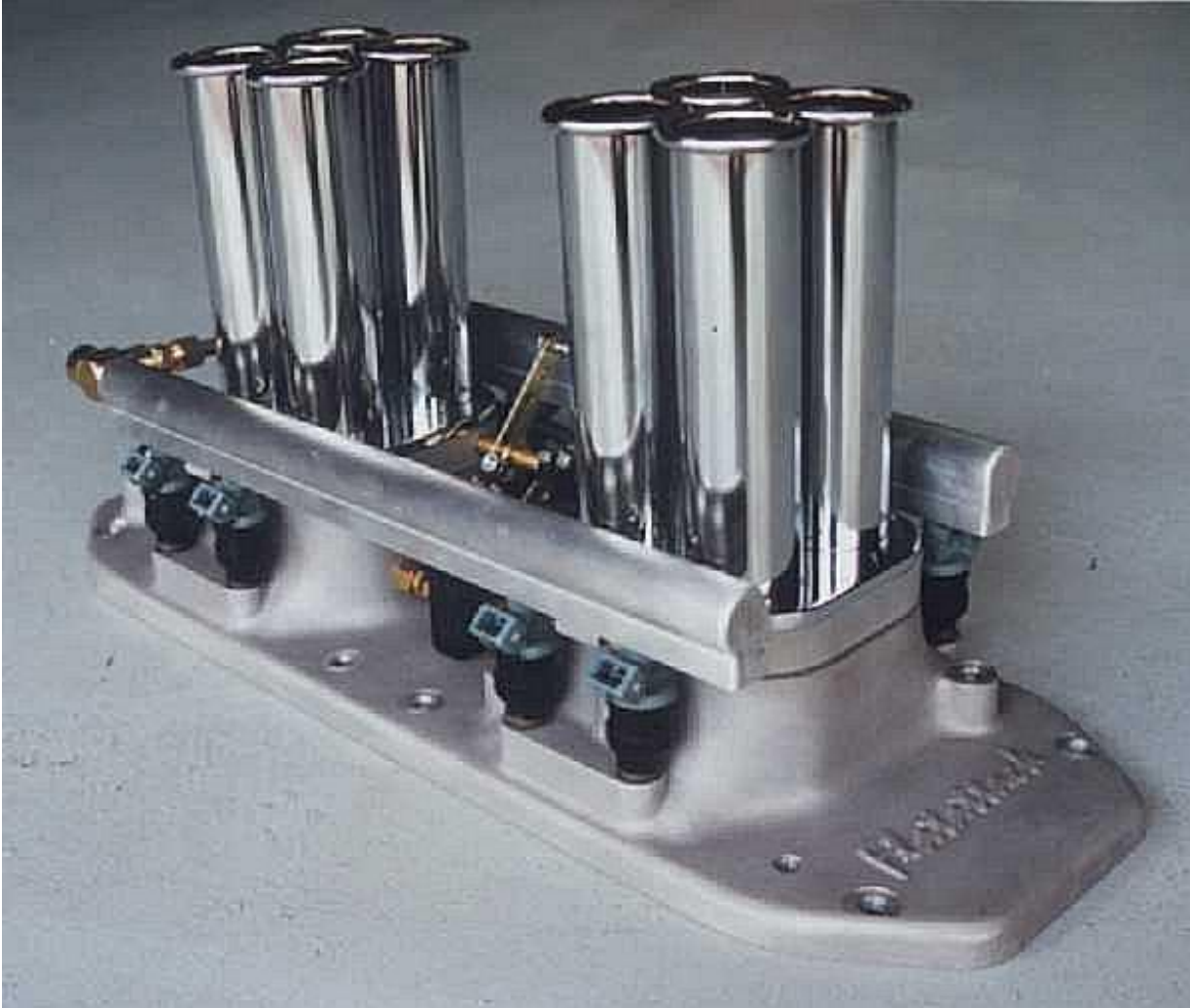
Figure 4 - Mike Davidson's (Flat Attack Racing) Hilborn style flathead EFI conversion
